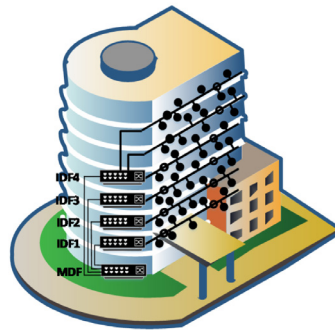
Figure 1. Typical placement of IDFs and MDF
